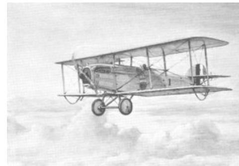
STANDARD MAIL PLANE, CURTISS JN4H, NEW YORK TO CHICAGO, 1918. Operator U.S. government; mail load, 180 pounds
